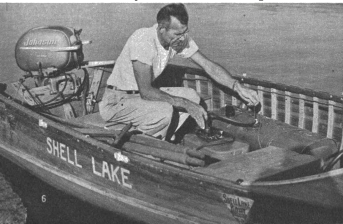
I used an old auto tank (cost me a buck) for my reserve supply of gas. Into it I installed an air pump from a discarded camp stove to force out the gas when needed.
