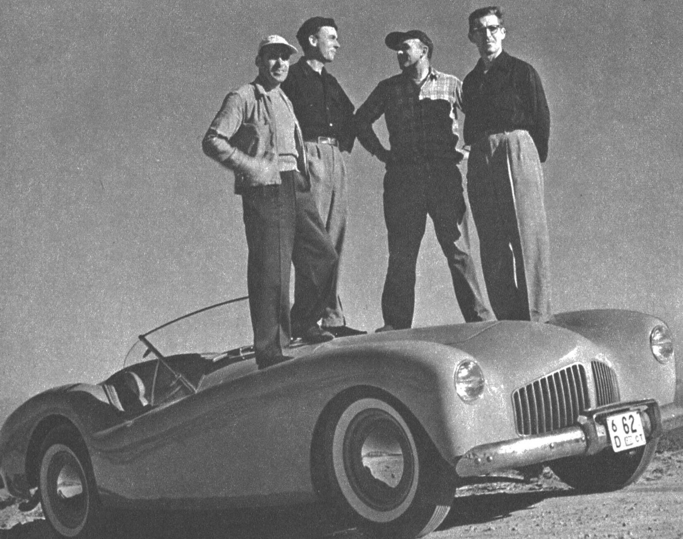
Four men stand on hood of Jaguar-like plastic auto body to demonstrate its strength. Made by the Glasspar Company of Costa Mesa, California.
